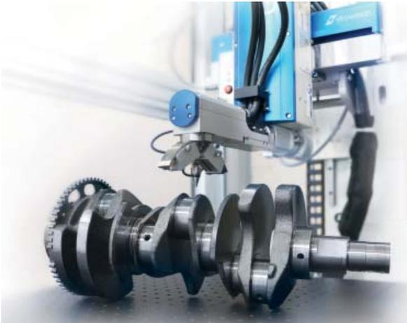
**Xstress 3000 G3 measures residual stresses on a crankshaft**
