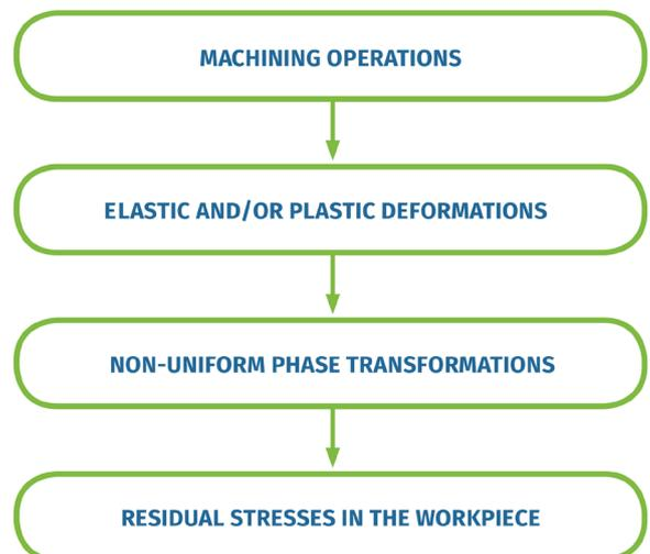
Thermal effects are created by the process causing a change in the dislocation density and distribution as well as surface integrity. In addition, pressure and the temperature of the cooling are important effects which contribute to formation of residual stresses.
