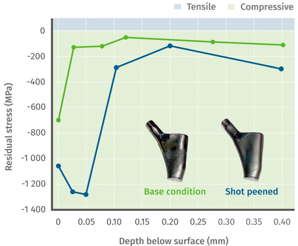
Shot peening has a place in many industries, including the health industry. The graph shows a Titanium hip joint's residual stress depth profile before the shot peening and after the shot peening. The process is applied to improve the hip joint's durability by creating higher compressive residual stresses on the surface and subsurface layers. The after-process graph shows that the aim is achieved.
