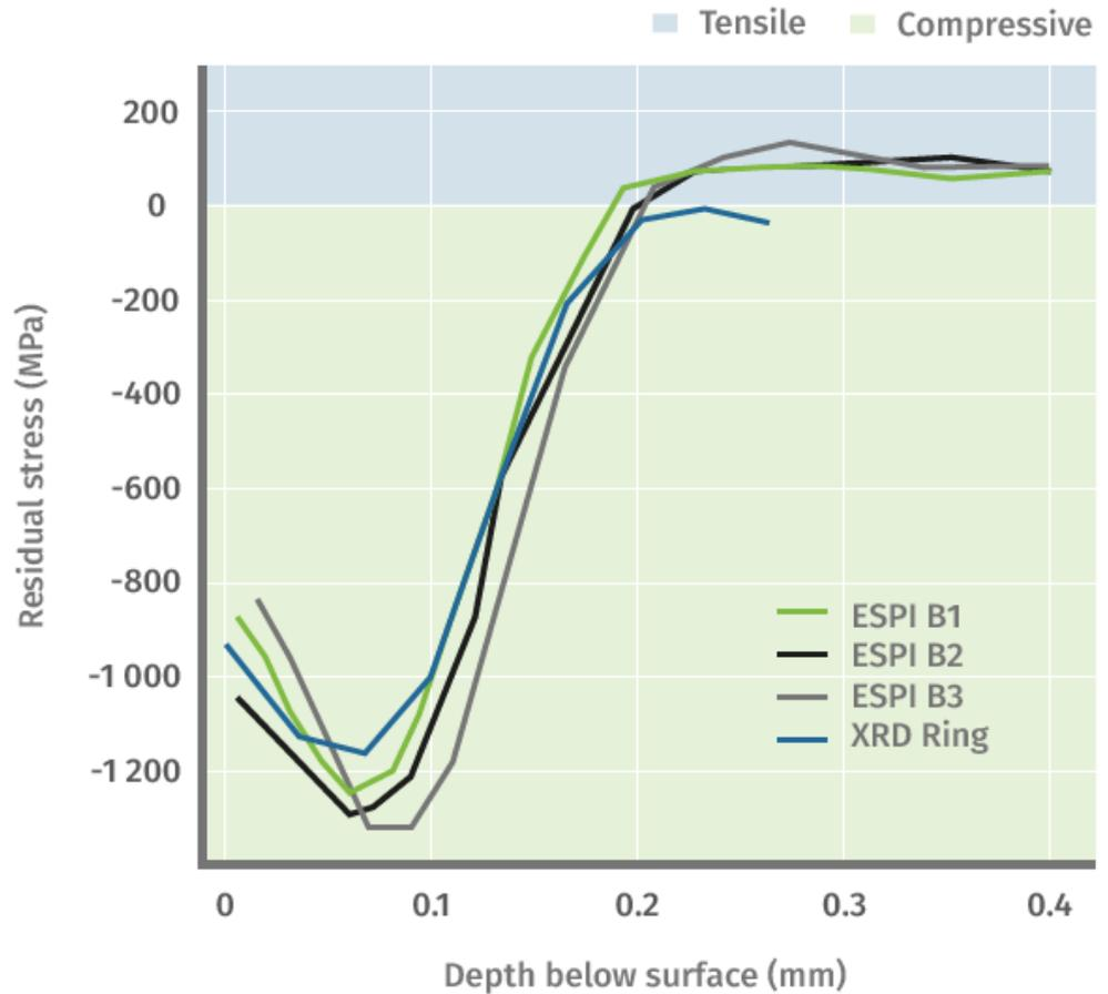
The graph shows four different stress depth profile of a shot-peened steel part. First, the part has been measured with X-ray diffraction (XRD Ring) and then consecutively three times with ESPI/Hole drilling technique (ESPI B1, B2, B3) to verify reliable and consistent results.
